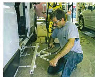
GYS aluminum/steel dent pulling system pulling a rocker straight on a van. Body tech pictured is Brian Aubuchon .
