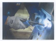
equipment fitted with ACT (automotive cold transfer) can weld as low as 32amps, which is perfect for these thin steels.
