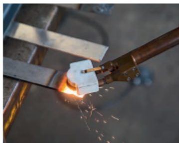
Right: Careful - sheet steel metal melts fast when too much heat is dialled in at the set.
