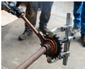
Bottom: Handy: a smaller ring inductor heated only the sprocket boss and not the shaft, so the sprocket pulled off easily.
