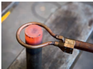
Top: GYS's ring inductors span diameters from 25-120mm, giving 360° heat input. Max power from the 220LG brought this 50mm shaft to workable heat in under three minutes.
