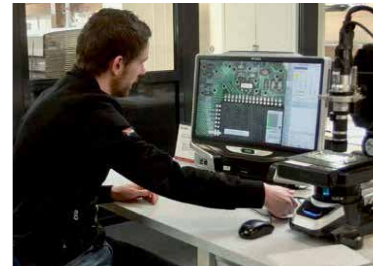
This microscope, which magnifies two thousand times, can be used to check micro-welds on electronic boards, for example.
