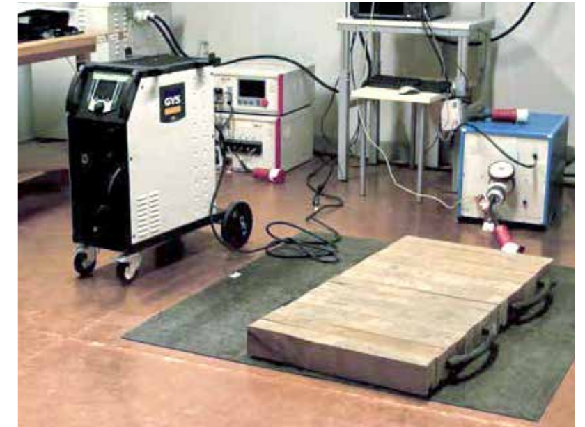
The prototype testing area has been expanded to streamline the process between design office projects, and the start of production. This copper floored area, in which the power source can be tested for electromagnetic interference, will be doubled in size.
