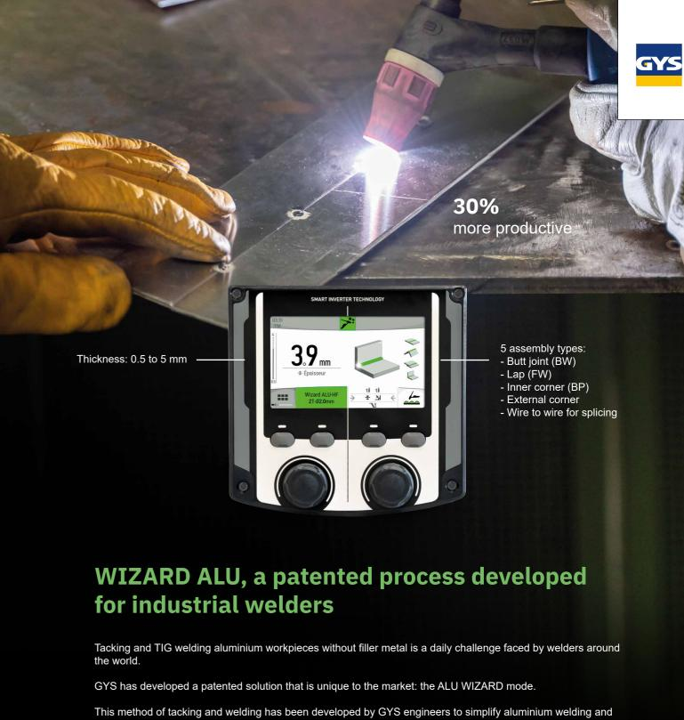
This method of tacking and welding has been developed by GYS engineers to simplify aluminium welding and make it accessible to everyone. With or without filler metal, this built-in feature of the TITANIUM range ensures that the tacking process takes less than a second. This mode is also available for tacking and welding all types of materials: steel, stainless steel, aluminium and copper.
